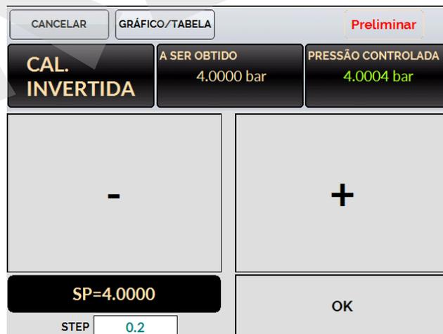
Fig. 67 - Inverted Calibration
