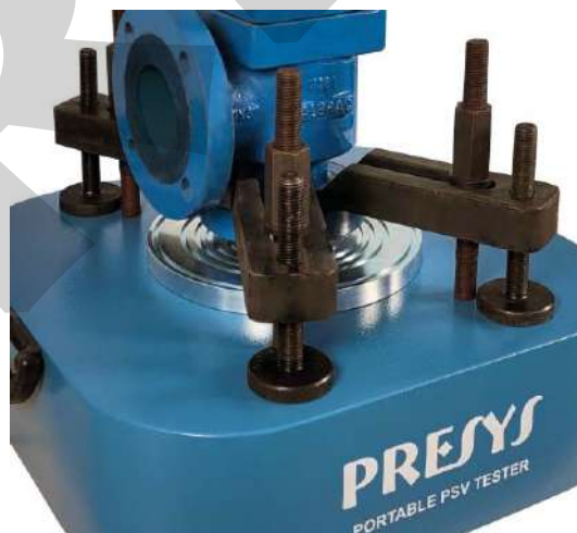
Fig. 22 - Valve fixed to the table
